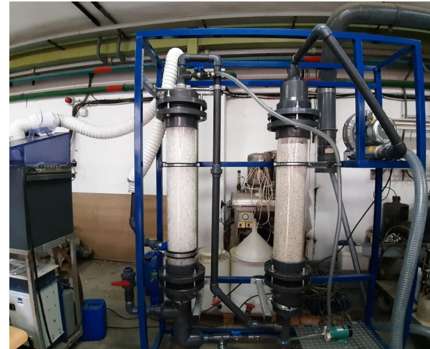
Wet scrubber: Packed bed absorber with pall rings + soda countercurrent
