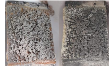
Sintering - Inert atmosphere - 400°C 2h
